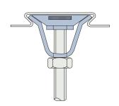
The Multiwedge 2 is designed for Multideck\* 60 and Multideck 80 profiles manufactured by Kingspan\* Structural Products (see page 56).
