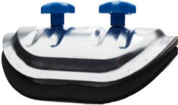
Curved Access Doors suitable for low, medium and high-pressure applications. Made from pressed steel with a zinc coating (Z275), they have two tightening knobs and a one-piece closed cell high density gasket to ensure the tightest possible seal when fitted.
